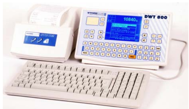
Step 8: Adjustment of the weighing indicator and test with reference weight (e.g. vehicle, weighing document print-out trial)
